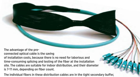
connected directly to the secondary buffer without the protective tubing. For this reason, these pre-terminated cables cannot be used repeatedly as 'multi-patch cords' for repeated direct connection to active elements - they are specifically designed for connections between optical distribution frames in data centers.
